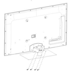
3 Secure the stand to your TV using the provided four M6  $\times$  12 screws.
